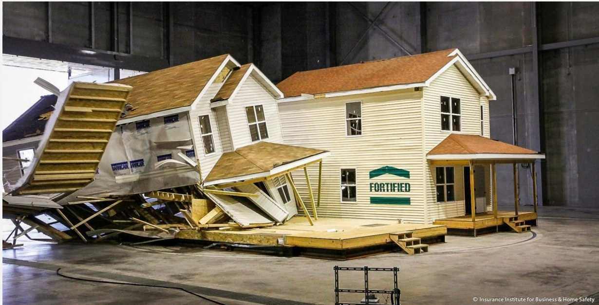
Image 1. Wind tunnel test of a house built with the Fortified construction standard. Source: Insurance Institute for Business & Home Safety [52].
