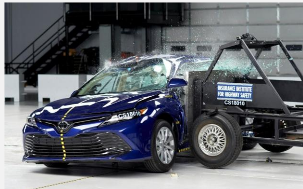
Images 2 and 3. From left to right: vehicle failing an Automatic Emergency Braking test; left-side crash test. Source: Insurance Institute for Highway Safety [198], [199].
