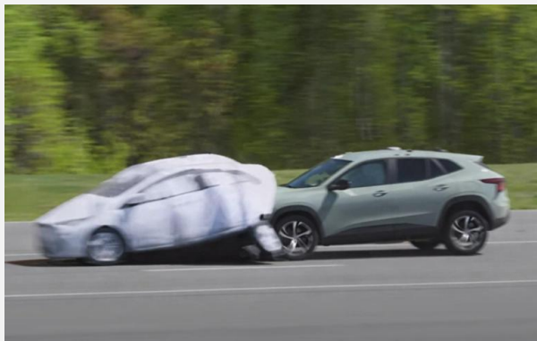
Images 2 and 3. From left to right: vehicle failing an Automatic Emergency Braking test; left-side crash test. Source: Insurance Institute for Highway Safety [198], [199].
